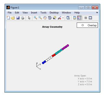
Each color other than white represents a different subarray. White represents elements that occur in multiple subarrays.
