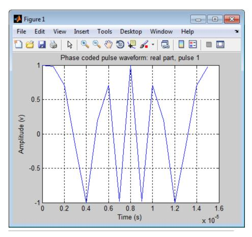
Generate samples of a phase-coded pulse waveform that uses the Zadoff-Chu code, and plot the samples.
