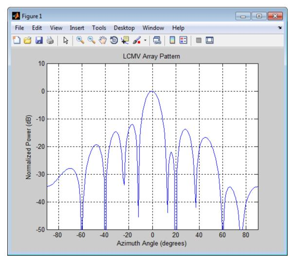
The above figure shows that maximum gain is attained at  $0^{\circ}$  as expected. In addition, the constraints impose nulls at  $-40^{\circ}$  and  $20^{\circ}$  and these can be seen in the plot. The nulls at  $-60^{\circ}$  and  $60^{\circ}$  arise from the fundamental property of the LCMV beamformer of suppressing the
