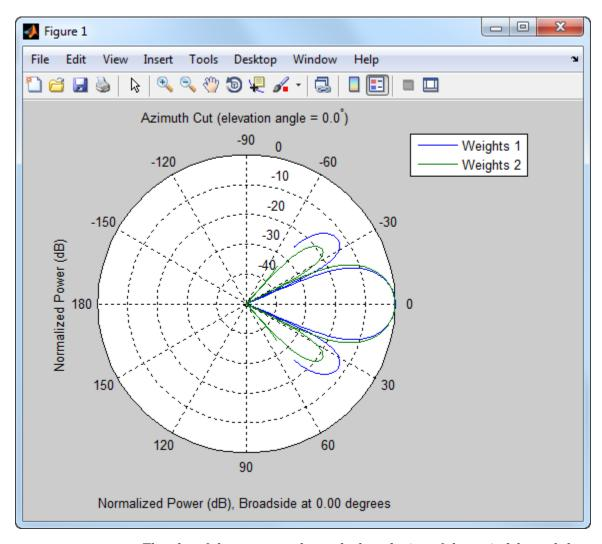
The plot of the response shows the broadening of the main lobe and the reduction of the strength of the sidelobes caused by the weight tapering.
