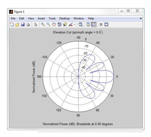
Construct a 24-element disk array using elements with two different antenna patterns. Plot the elevation response of this array using uniform weights on the elements and also a tapered set of weights set
