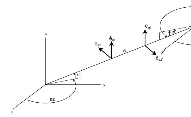
The polarization loss is the projection (or dot product) of the normalized transmitted field vector onto the normalized receiver polarization vector. Notice that the loss occurs because of the mismatch in direction of the two vectors not in their magnitudes. Because the vectors are
