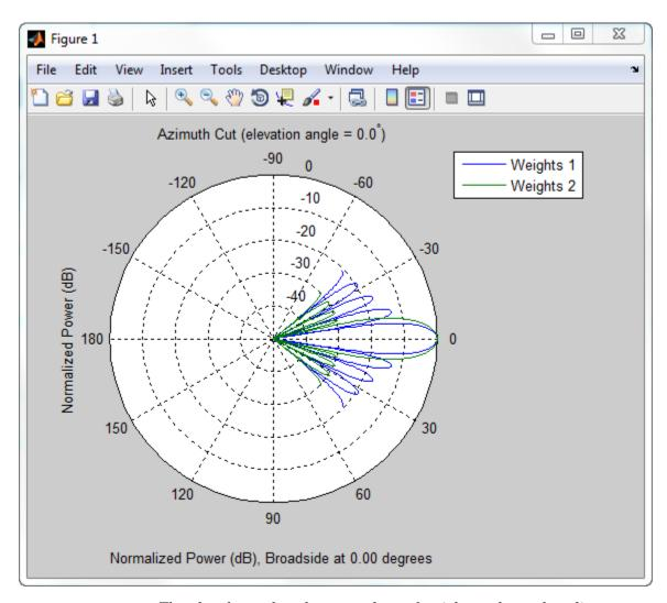
The plot shows that the tapered set of weights reduces the adjacent sidelobes while broadening the main lobe.
