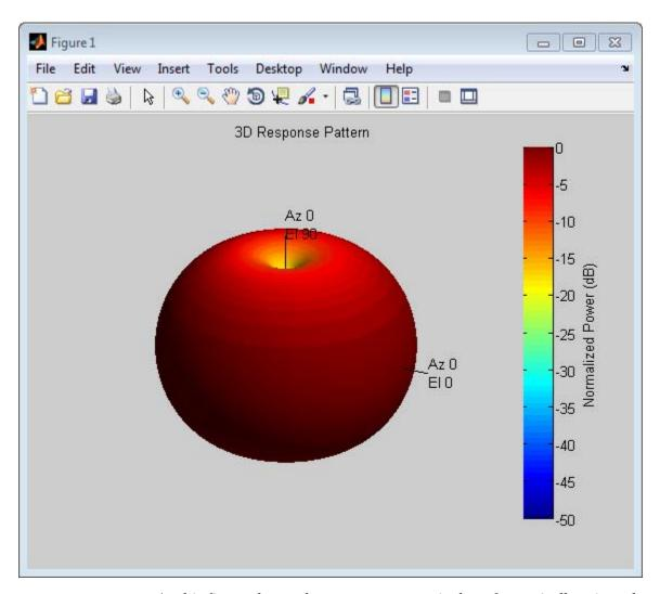
As this figure shows, the antenna pattern is that of a vertically-oriented dipole and has its maximum at the equator and nulls at the poles.
