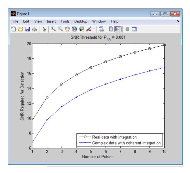
Plot the linear detection threshold against the number of pulses, for real and complex data. In each case, the threshold achieves a probability of false alarm of 0.001.
