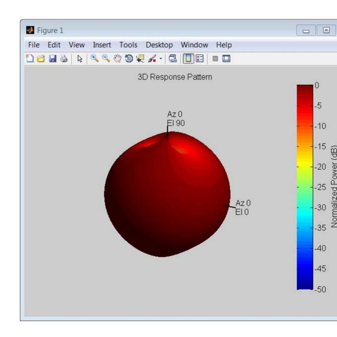
The antenna pattern of the horizontal-polarization also has maxima at  $\pm 0^{\circ}$  elevation and  $\pm 0^{\circ}$  azimuth but no response at  $\pm 90^{\circ}$  azimuth as shown in this figure.
