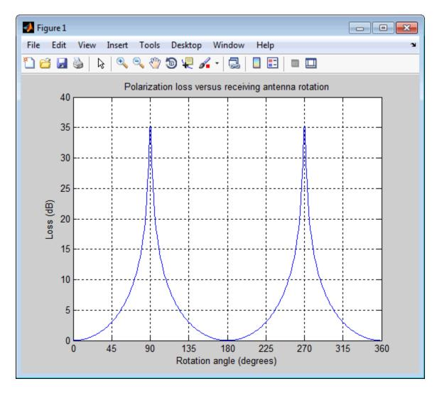
The angle-loss shows nulls (Inf dB) at 90° and 270° where the polarizations are orthogonal.
