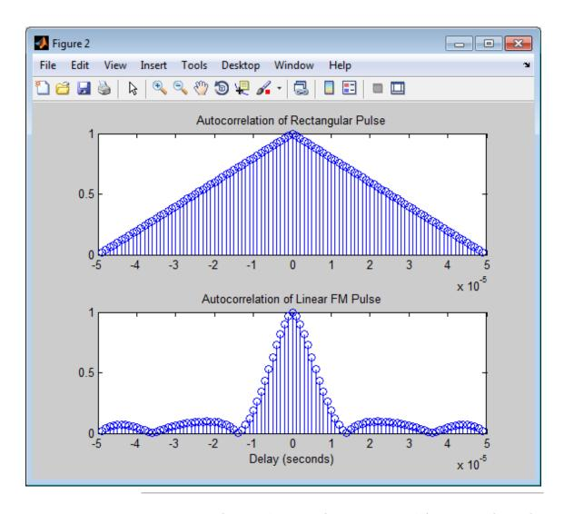
Nonzero-Doppler cuts (autocorrelation sequences) for rectangular and linear FM pulses of the same duration. Both cuts were taken at a 5 kHz Doppler shift. Besides the reduction of the peak value, there is a strong
