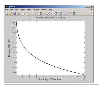
Compute the required SNR for 10 noncoherently integrated samples as a function of the false-alarm probability with the probability of detection equal to 0.9.
