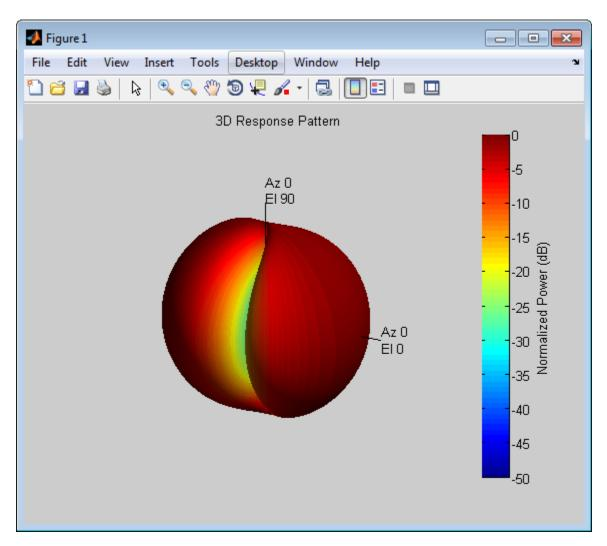
This figure shows the vertical polarization response.
