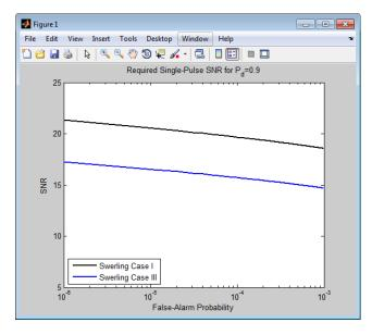
Note that the presence of a dominant scatterer reduces the required SNR for the specified detection and false-alarm probabilities.
