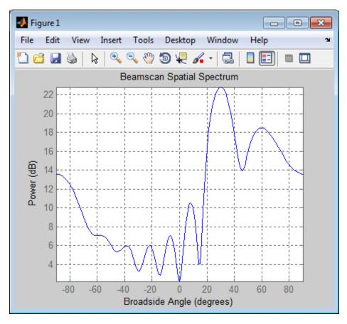
The plot shows a high peak at 30 degrees and a lower peak at 60 degrees.
