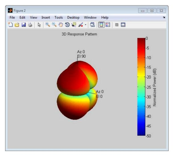
This combined response best illustrates the polarity of the short-dipole.
