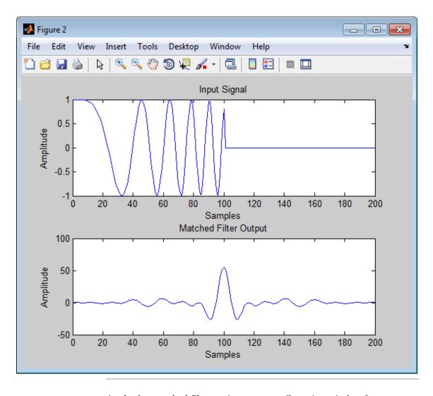
Apply the matched filter, using a custom Gaussian window for spectrum weighting.  $\,$
