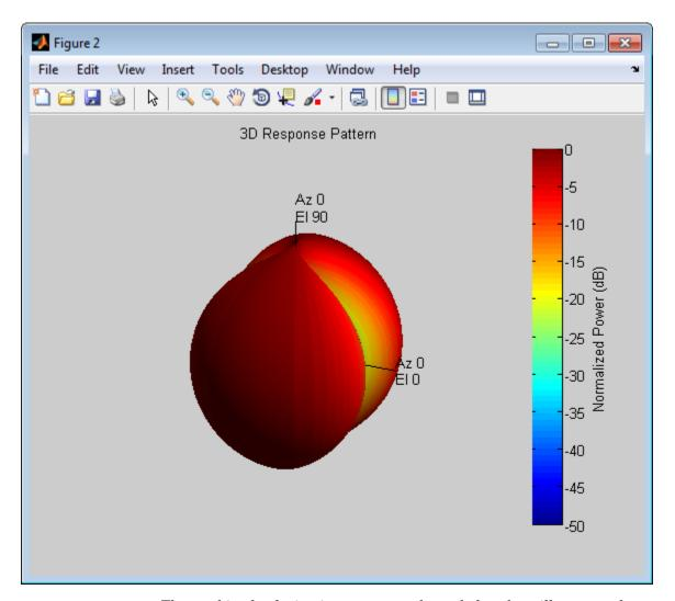
The combined polarization response, shown below, best illustrates the x-axis polarity of the dipole.
