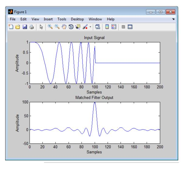
Apply the matched filter, using a Hamming window to do spectrum weighting.
