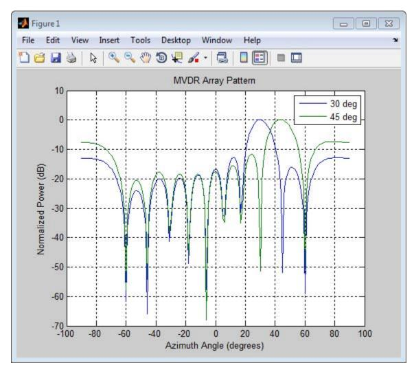
The figure shows plots for each beamformer direction. One plot has the expected maximum gain at 30° and the other at 45°. The nulls at -60° and 60° arise from the fundamental property of the MVDR beamformer in suppressing power in all directions except for the arrival direction.
